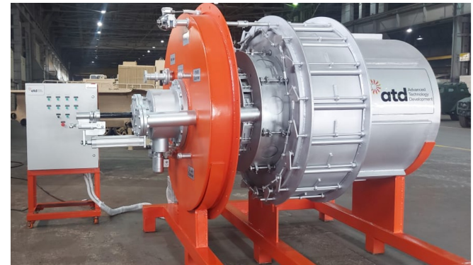
The new HEAT burner system (53 MW)
